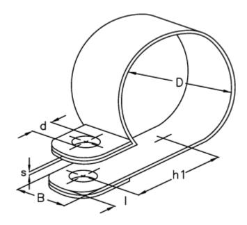
$\begin{array}{ll} d & = 4.3 \\ \text{Diameter D} = 9 \\ \text{h1} & = 9.2 \\ \text{I} & = 3.8 \\ \text{s} & = 0.4 \\ \text{Width B} & = 9 \\ \end{array}$
